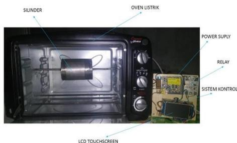
Gambar 9. Tampilan thermal milling machine
